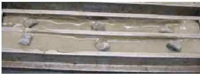
Figure 1 – Two cement paste bars containing sulphides aggregates
